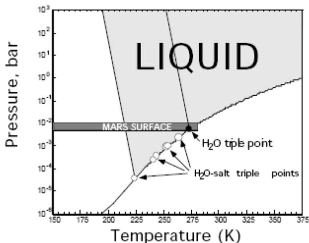
Fig. 2. P-T diagram showing the stability field for liquid brines, compared to the estimated temperature-pressure conditions on the martian surface (shaded horizontal box). Note that much of the range of surface P-T conditions falls within the liquid field.
